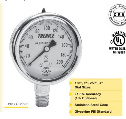
The Trerice **D80 Series** Industrial Gauge is designed for rugged performance requirements at an economical cost. This liquid filled gauge is furnished with a stainless steel case and crimped ring. Wetted parts are either bronze tube with Lead-Free (PBF) brass socket or stainless steel.
